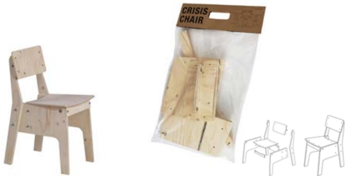
**CRISIS CHAIR** The crisis concept is based on the ring, nut and bolt, where the nut becomes locked inside the ring hole. Since the plywood is not strong enough to make long thin legs, the sides are made of relatively large pieces of plywood. It is these large surfaces that give the crisis chair its own unique character and allow for the possibility to work with bold colours. It seems that every time a crisis looms, sales of the entire crisis collection start picking up.
